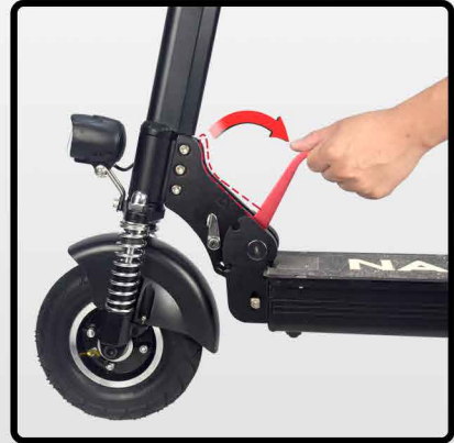
① Pull the red folding stick in the direction of the arrow
