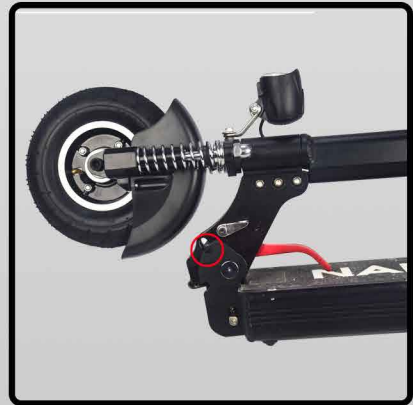
③ When the black post is caught in the upper slot, the folding is completed.
