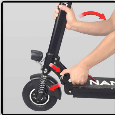
② Press the silver snap in the direction of the arrow so that the black post completely leaves the lower slot and lower the pole in the direction of the arrow
