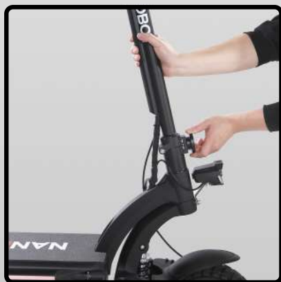
③ Make sure to perfectly align the J -shaped buckle.
